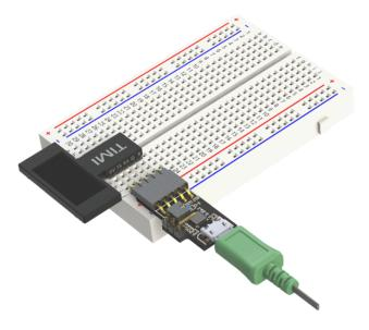
The Mates Programmer can also be directly connected to the appropriate row of 5 male pins on BBM products such as TIMI-96 if direct programming is desired instead.
